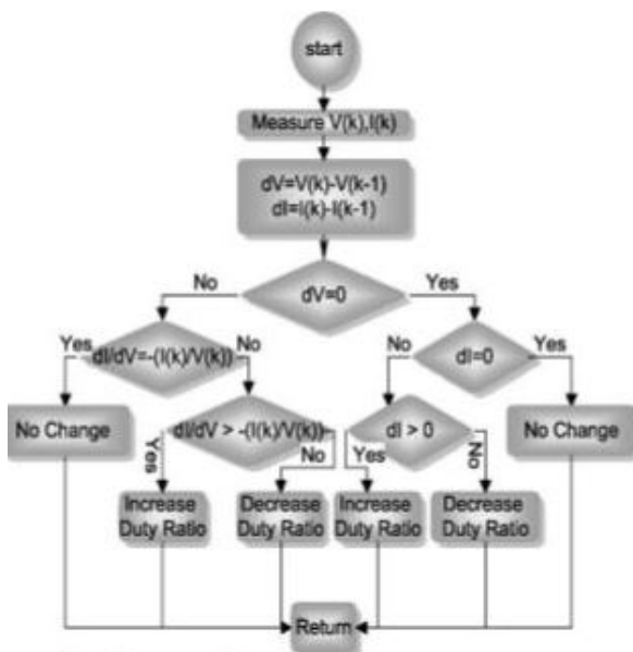
Figure 5: Flow chart of Incremental Conductance (INC) algorithm
